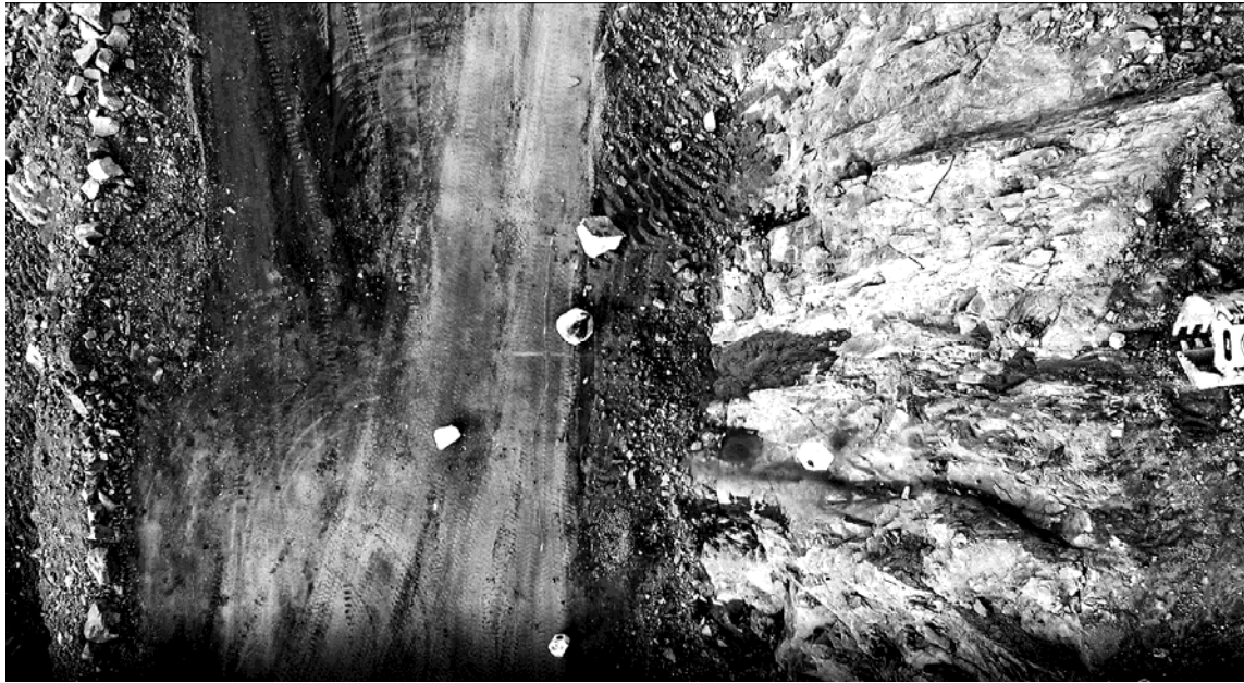
Fig. 2 Drop tests in a granite quarry at Limberg, Lower Austria. Geological unit of the Bohemian Massif. Monitoring with the aid of a video recording drone.
